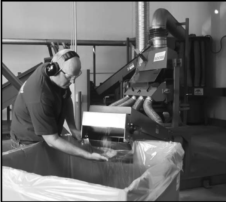
Separator SE 40 as part of the POWERCAT cable recycling plant.
