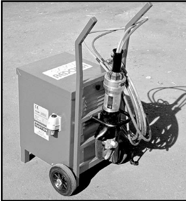
Enclosed hydraulic power unit and cutter.
