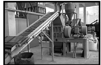
Granulator with transport equipment.
