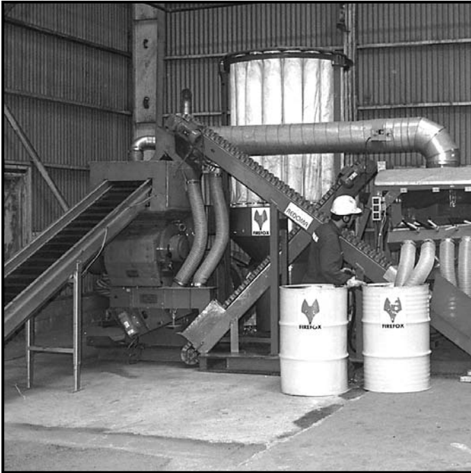
Granulator GR 45 (left) as part of a FIREFOX Cable Recycling Plant.
