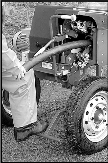
Feeding a power cable into the stripper.
